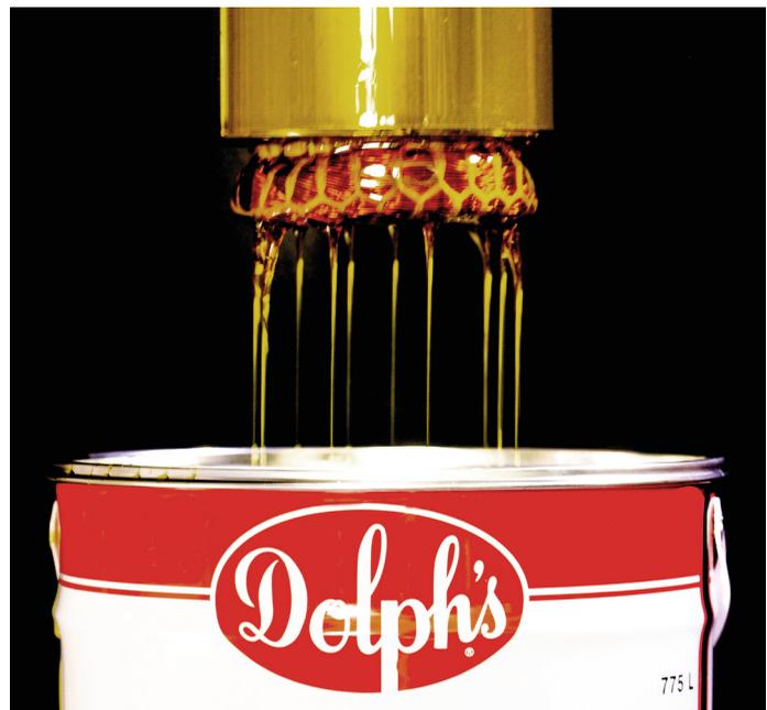
Dipping process for stator impregnation.
